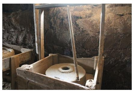
The process of cracking open our grain to expose and crush the grain. This exposes the endosperm, which leads to higher efficiencies (more starch).
